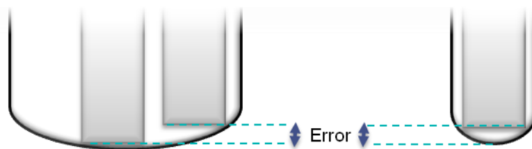
Figure 28 - Error in Bore Depth Measurement
