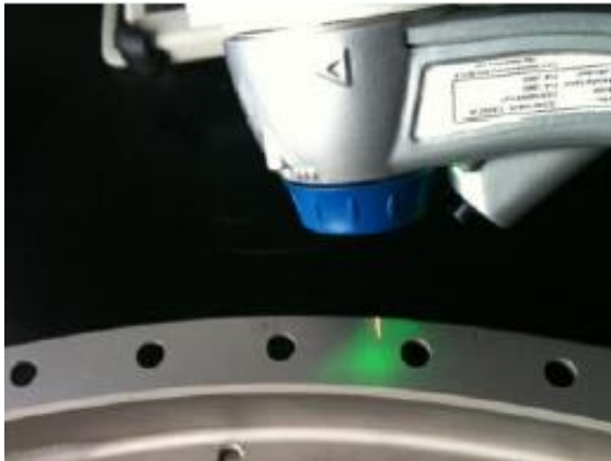
Figure 79 - GapGun Scanning a Radius
