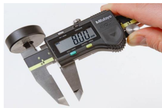
Figure 19 - Checking Anvils with Gauge Block Figure 20 - Checking Anvils with Setting Ring (Mitutoyo UK Ltd)
