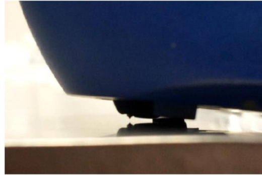
Figure 73 - Curvature causing stylus to leave surface
