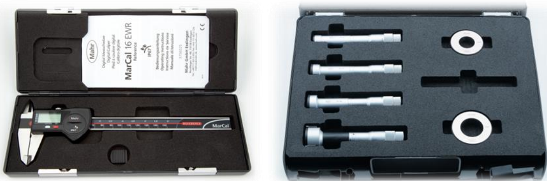
Figure 6 - Good gauge storage practice (Rolls-Royce & Mahr)
