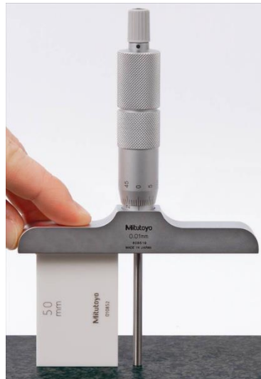
Figure 27 - Checking Depth Micrometer with Gauge Block (Mitutoyo UK Ltd)
