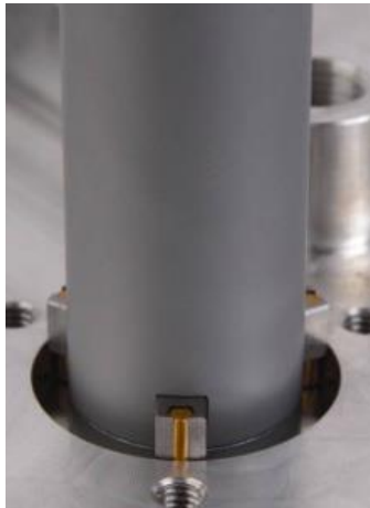
Figure 36 - 3 Point Bore Micrometer self-aligning in hole (Mitutoyo UK Ltd)
