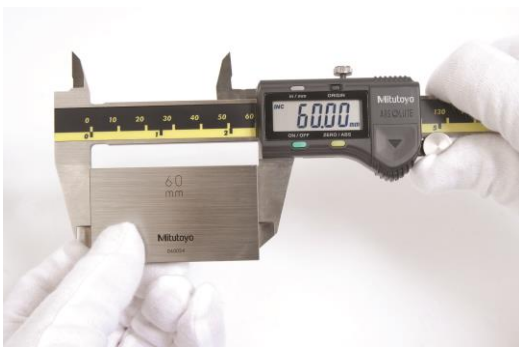
Figure 19 - Checking Anvils with Gauge Block Figure 20 - Checking Anvils with Setting Ring (Mitutoyo UK Ltd)
