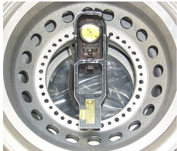
Figure 53 - Omnigauge Measuring a Disk Bore
